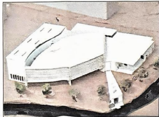
Magen Dean brings natural light into her gallery design with 'light shelves' on three walls and a curving interior wall rising above the roof to capture daylight.
