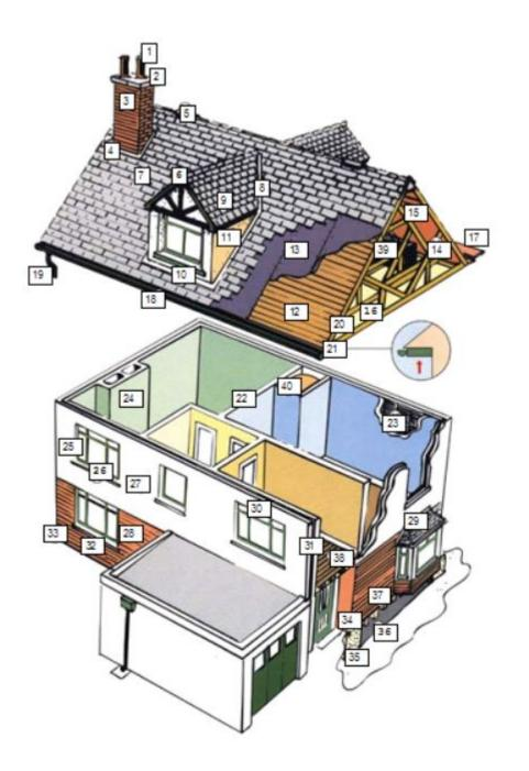
3 Chimney head Flashing 4 Ridge ventilation 5 Ridge board Slates/tiles 8 Valley guttering 9 Dormer projection Dormer flashing 10 Dormer cheeks 11 12 Sarking Roof felt 13 Trusses 14 15 Collar 16 Insulation 17 Parapet gutter Eaves guttering 18 Rainwater downpipe 19 20 Verge boards / skews 21 Soffit boards 22 Partition wall Lath / plaster 23 24 Chimney breast 25 Window pointing Window sills 26 Rendering 27 Brickwork / pointing 28 Bay window 29
